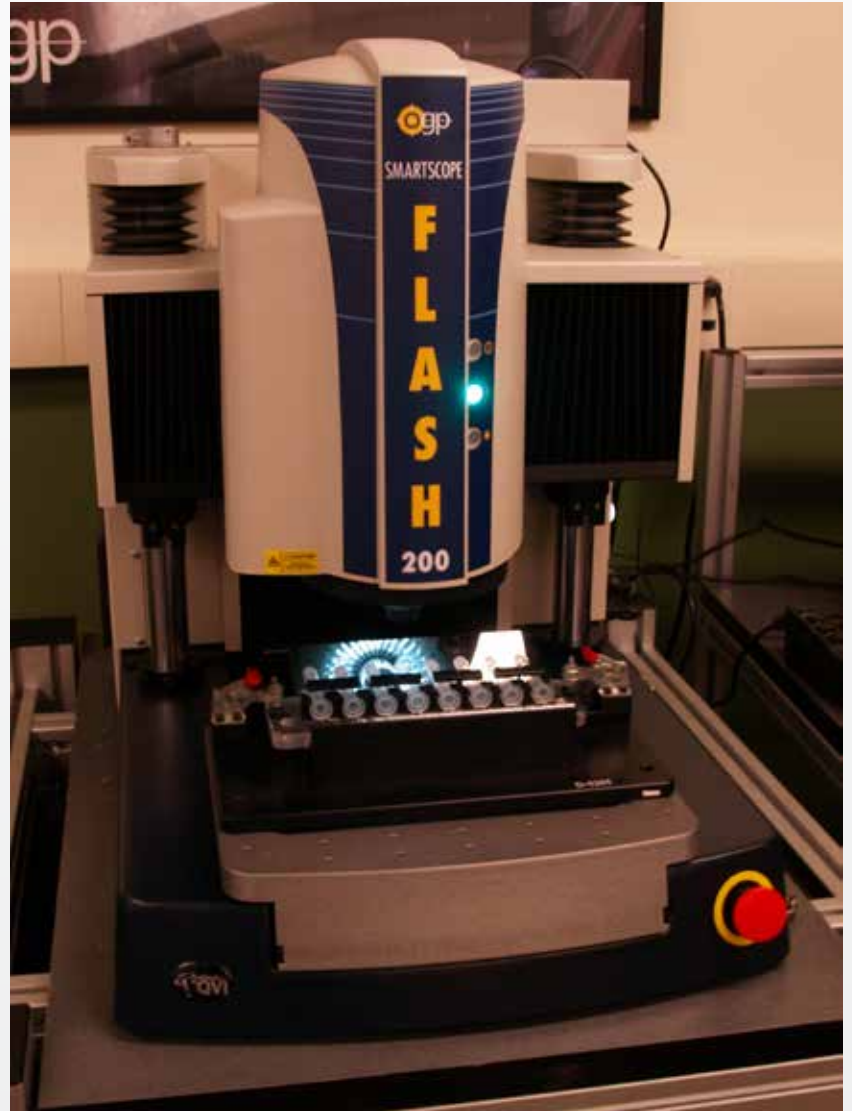
Eight syringes on a custom gang fixture.
